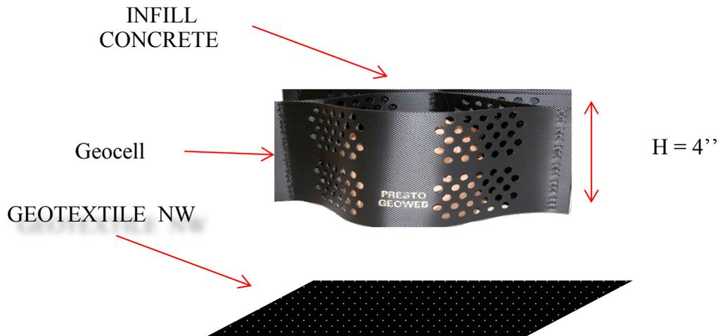
Figure 1. Concrete Infill Geocellular Confinement System Scheme. Perforations shown should be 19% - 28% of total strip area.
