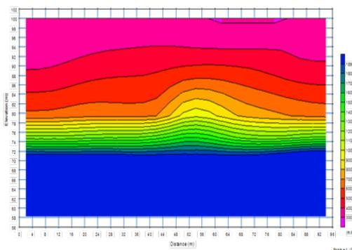
Figure N° 05. P-wave velocity seismic profile of seismic refraction test
