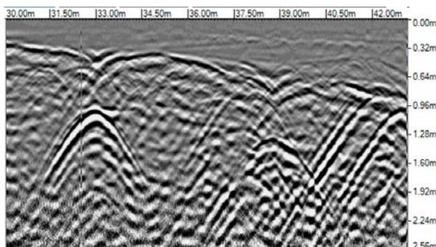
Figure N° 06. The radargram shows the anomaly is in form of parabola
