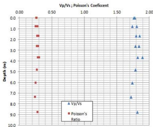
Figure N°07 Vp/Vs Ratio and Poisson's ratio with the depth
