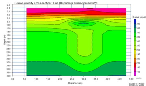
Figure N° 04. S-wave velocity seismic profile of MASW test
