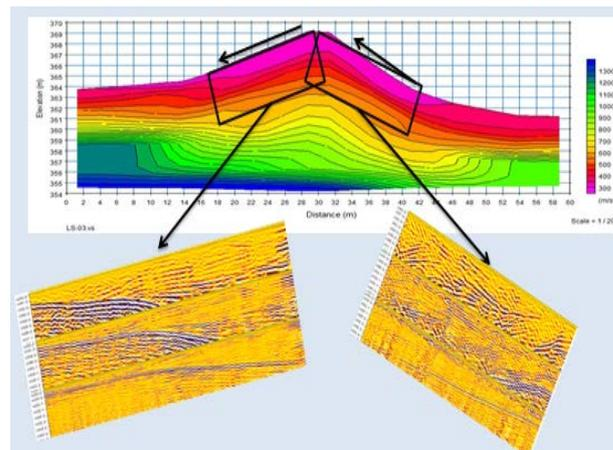
Figure N° 03. Evaluation of thickness of the aeolian sand of the dune by compare the seismic profile and radargram
